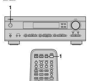
1 Press STANDBY/ON (SYSTEM POWER on the remote control) to turn on the power of this unit.
