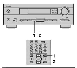
1 Press A/B/C/D/E (A/B/C/D/E on the remote control) to select the preset station group.
